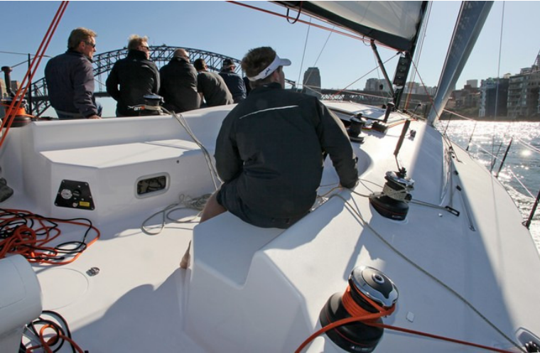
The shallow coachroof design permits close sheeting of the jib and clean leads for the barber haulers - Sydney Yachts GTS43
